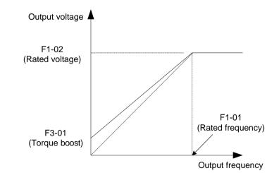
Output voltage and output frequency change linearly when below rated frequency. It is applicable to general mechanical drive applications such as conveyors where the load torque is constant against the speed range.
