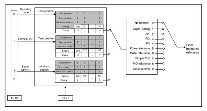
Figure 6-29 Command source + main frequency reference setting channel
