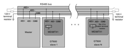
It is recommended to use an STP cable as the RS485 bus and use a twisted cable to connect 485+ and 485-. Connect a matching terminal resistor of 120  $\Omega$  respectively at both ends of the bus to prevent signal reflection. The RS485 bus allows connection of a maximum of 128 nodes and the distance of each node branch must be smaller than 3 m. Connect the reference ground of all nodes together.
