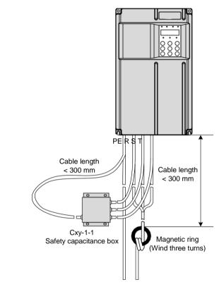
Mounting dimensions of filter capacitance box
