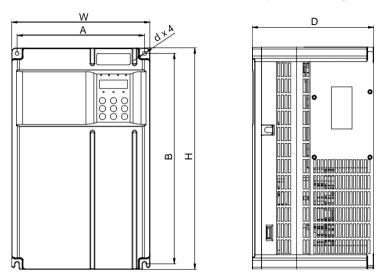
Figure 2-6 Overall dimensions of GT600-4T45GB to GT600-4T160G (sheet metal housing)
