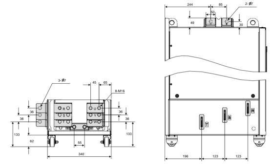
Figure 3-12 Terminal dimensions of GT600-4T315G/450G (without output reactor)
