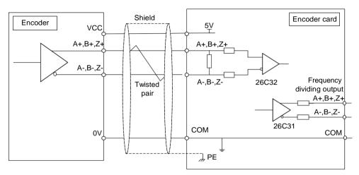
Grounding Shield of Extension Encoder Card
