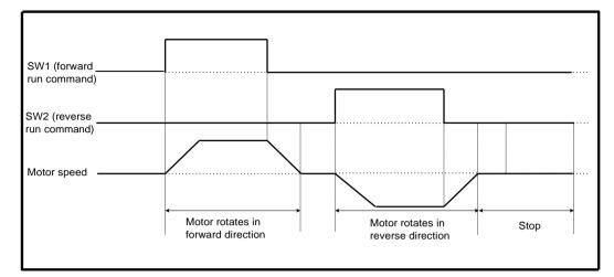
Figure 6-3 Two-wire 1 sequence (normal)
