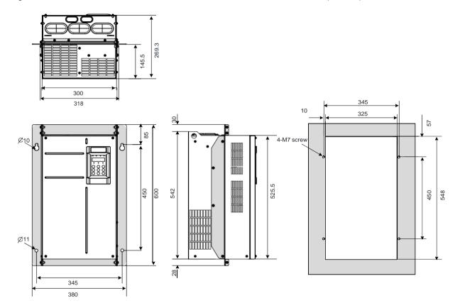
Figure 8-3 Bracket dimensions and hole size of GT600-4T45GB to GT600-4T55GB (unit:mm)
