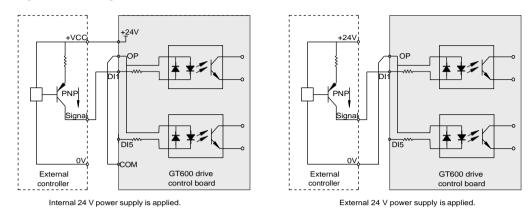
If you intend to use internal power supply of the drive, remove the jumper between terminals +24V and OP. Connect +24V to the common port of external controller, and connect terminal OP to terminal COM.
