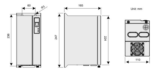
Always mount MDBUN series braking unit in an upright position.
