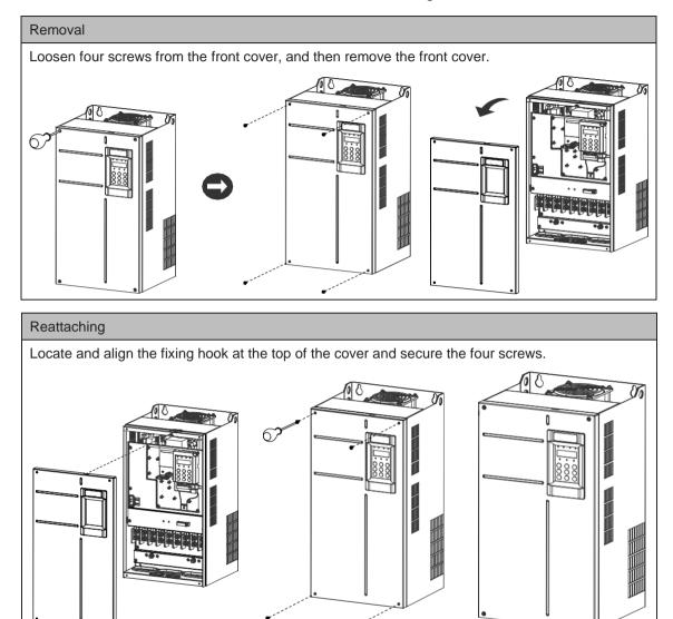
Remove and Refit the Front cover of a Sheet Metal Housing
