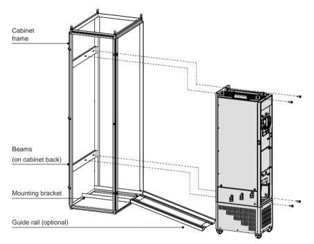
• Check that installation of the drive is secure and remove the guide rail.
