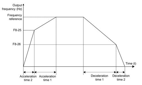
During acceleration, if the running frequency is below F8-25, acceleration time 2 is selected. If it is above F8-25, acceleration time 1 is selected.
