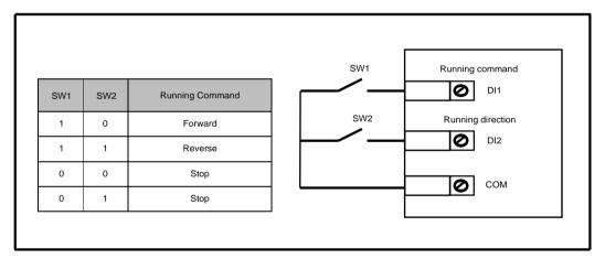
Sequence diagram of two-wire control mode 2 is shown in the following figure.
