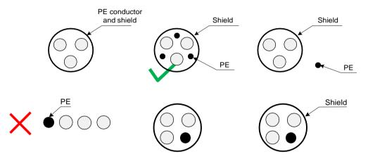
To suppress emission and conduction of radio frequency interference effectively, shield of cable is cooper braid. Braided density of cooper braid should be greater than 90% to enhance shielding efficiency and conductivity, as shown in the following figure.
