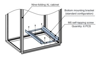
• Assemble the guide rail (model: GT600-AZJ-A3T10, optional).
