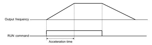
Figure 6-30 (2) Sequence of start with start frequency
