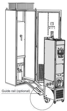
• Push the drive into the cabinet slowly. Please use auxiliary strap in the process of push-in to prevent turnover, as shown in the following figure.
