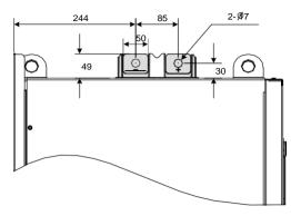
Figure 3-14 Terminal dimensions of GT600-4T315G-L/450G-L (without side entry copper bar, without output reactor)
