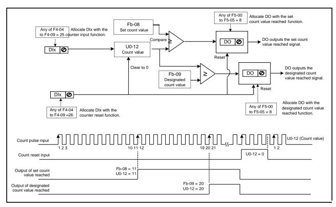
The settings of related function parameters in the preceding figure are as follows:
