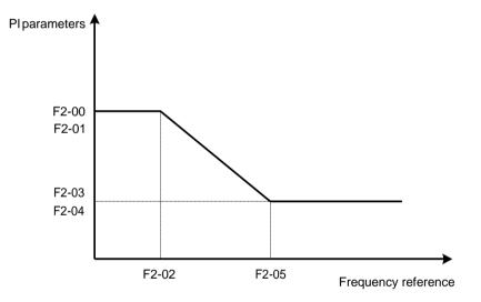
To improve the system response, increase the proportional gain or reduce the integral time. Remember to increase proportional gain first to ensure that the system does not oscillate, and then reduce integral time to ensure that the system has quick response and small overshoot.
