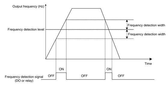
The drive provides two groups of frequency detection parameters for the digital output functions 26 and 27. When the output frequency is in the range of the detection width, the digital output terminal set for function 26 or 27 becomes on.
