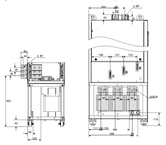
In Figure 3-13, the side entry copper bar can be removed if necessary. Terminal dimensions of main circuit terminals without side entry copper bar are shown below.
