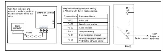
When the AC drive is controlled via communication, host computer must send write command to the AC drive. Here takes Modbus as an example to describe process of giving RUN command via serial communication.
