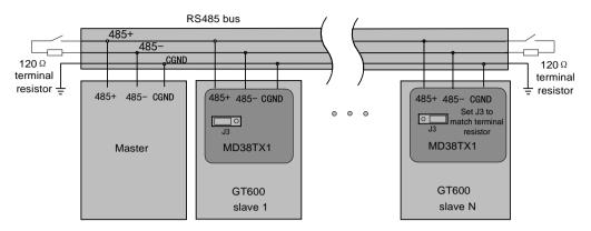
It is necessary to connect a matching terminal resistor to the end of PROFIBUS bus and set DIP switch properly. The system PEs must be reliably grounded.
