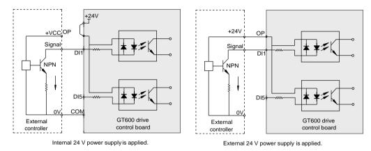
Applying internal 24 V power supply is the most commonly used wiring mode. In this mode, short terminals +24V and OP and connect COM to external power 0V.
