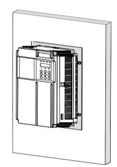
Through hole installation of a sheet metal housing
