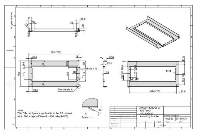
Figure 8-7 Bracket dimensions and hole size of GT600-4T250G(-L) to GT600-4T280G(-L) (unit: mm)
