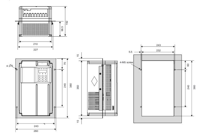
Figure 8-2 Bracket dimensions and hole size of GT600-4T30GB to GT600-4T37GB (unit:mm)
