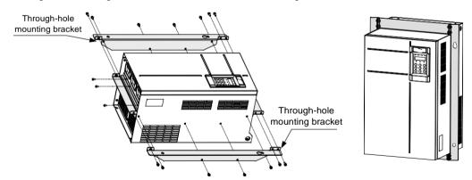
• Ensure all screws and bolts that secure the brackets to the housing are tight.
