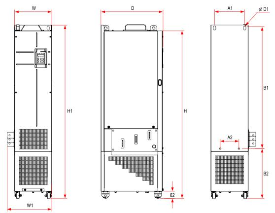
Figure 2-8 Overall dimensions of GT600-4T200G-L to GT600-4T450G-L
