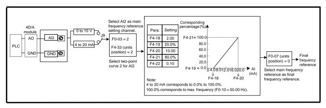
Figure 6-17 Current input at AI2 to control frequency reference
