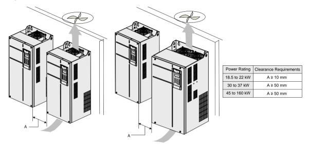
Where an AC drive is required to be mounted directly above another AC drive, it is recommended to install an Air Guide Plate to divert exhaust cooling air of the bottom unit away from the top unit.
