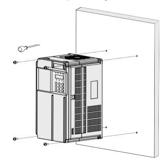
Figure 2-9 Backplate-mounted installation of a plastic housing
