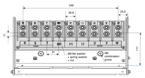
Table 3-4 Recommended cable dimensions and tightening torque of GT600-4T45GB/GT600-4T55GB
