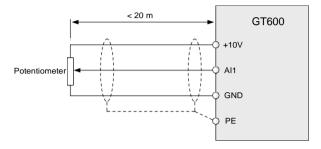
In applications where analog signals suffer from effects of severe external interference, install a filter capacitor or a ferrite magnetic core at source of analog signal. The pig tail of the shield must be connected to the PE terminal on the drive.
