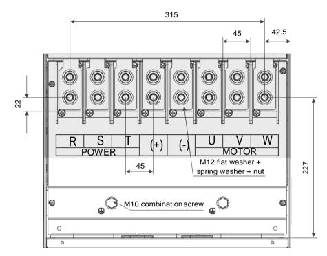
Figure 3-5 Terminal dimensions of GT600-4T132G/GT600-4T160G
