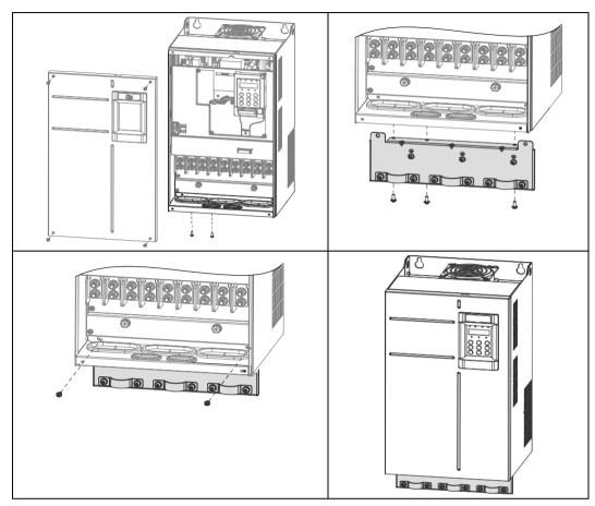
The Cable Support Bracket is an optional accessory which provides mechanical support for input, output and dynamic brake cables and which also provides grounding clamps for the screen/shield of the cables. Installation of the bracket is shown below.
