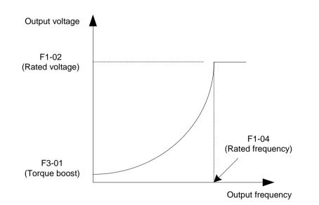
Output voltage and output frequency change according to square curve when below rated frequency. It is applicable to applications such as centrifugal fans where the load is inversely proportional to the speed.
