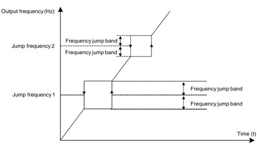
In the preceding figure, when running frequency accelerates to the value that is close to jump frequency during acceleration, the AC drive runs for a period at current frequency reference and then jumps over jump frequency. The jump width is twice of F8-11.
