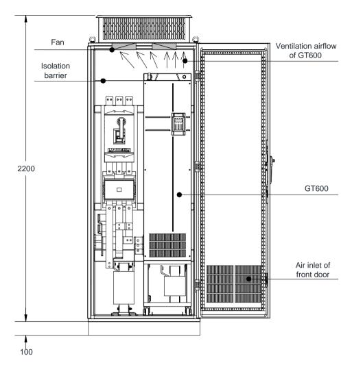
Figure 2-12 Cabinet with fan on the top
