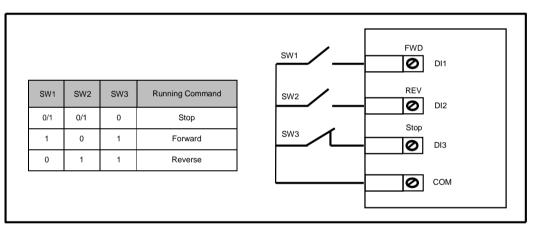
Sequence diagram of three-wire control mode 1 is shown in the following figure.
