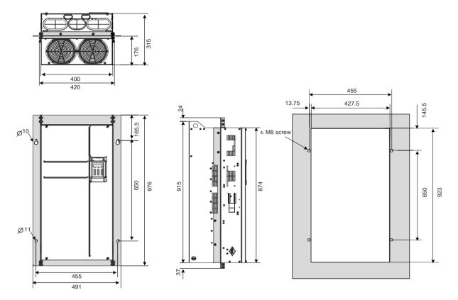
Figure 8-6 Bracket dimensions and hole size of GT600-4T200G(-L) to GT600-4T220G(-L) (unit: mm)
