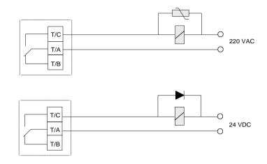
Figure 3-27 Wiring of relay
