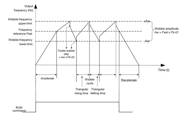
Figure 6-49 The wobble function schematic diagram
