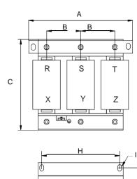
Dimensions of AC reactor of 490 to 660 A are shown as below:
