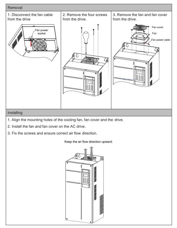
Removing and Installing the Fan of GT600-4T200G(-L) to GT600-4T450G(-L)
