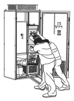
• Fix the AC drive to the beams on the back of the cabinet, as shown in the following figure.
