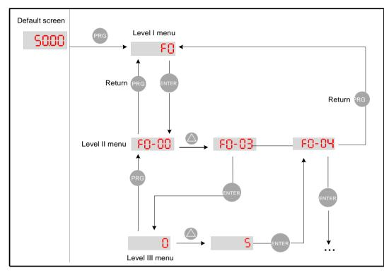
Operation procedure of the three levels of menu is as follows:
