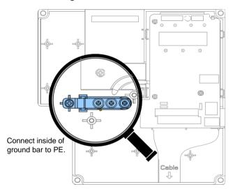
After installation of the PG card is done, PE of PG card is connected automatically. When connecting encoder, connect shield of signal lines to PE of PG card to complete the shield grounding.
