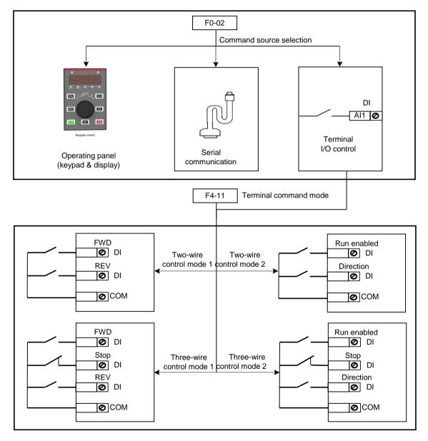
The following example takes DI1, DI2 and DI3 to describe how to control the AC drive via DI terminals.
