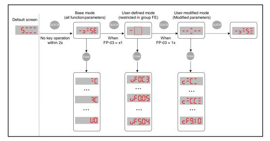
The value you set for function parameter FP-03 determines whether the operating panel displays quick-view user-defined and quick-view user-modified function groups. The base mode is always displayed.
