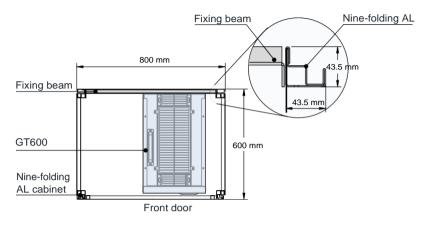
When the drive of GT600250G(-L) to GT600450G(-L) is mounted in the nine-folding AL cabinet of 600 mm deep, the fixing beam must fold inwards. When the drive is mounted in the cabinet of 800 mm deep, folding inwards is not required.
