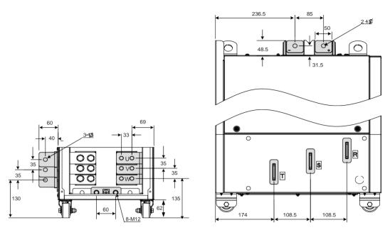
Figure 3-6 Terminal dimensions of GT600-4T200G/220G (without output reactor)
