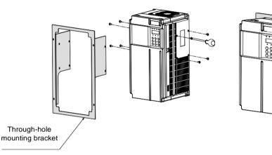
Through-hole mounting bracket installation for a sheet metal housing
