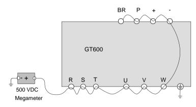
The measured insulation resistance must be greater than 5 M $\Omega$ .
