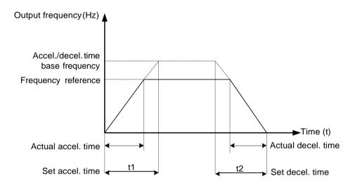
The AC drive provides totally four groups of acceleration/deceleration time for selection. You can perform switchover by using a DI terminal.
