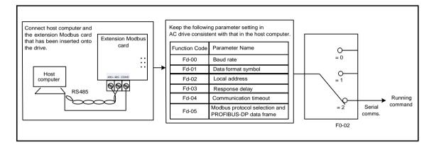
To make the drive run in reverse direction, the host computer sends the write command 01 06 20 00 00 02 03 CB (hexadecimal). In the command,
